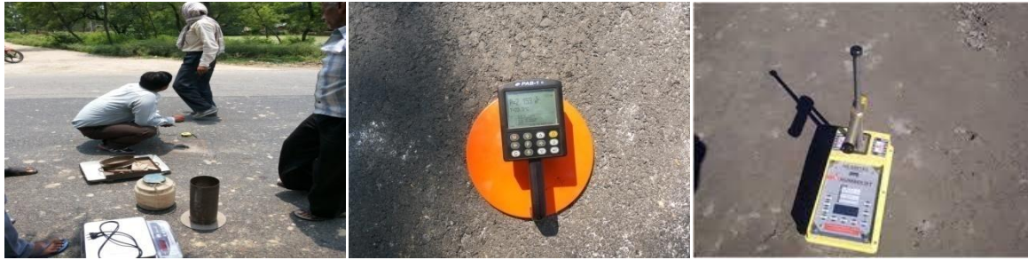
Figure 03: Sand Replacement Equipment, Nuclear Density Gauge (HUMBOLDT) and Non-nuclear Density Gauge (PAB1)
