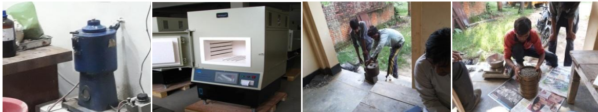
Figure 04: Bitumen Extraction, Bitumen Content Furnace and Gradation of (RAP)
