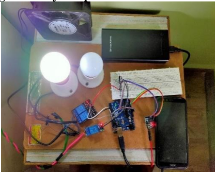
Figure 8 Key 4 is pressed and device 1 is OFF
