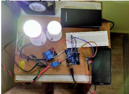
Figure 7 Key 2 is pressed and device 2 is ON
