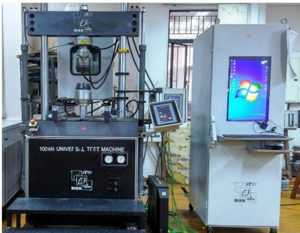
Fig. 2. BiSS Universal testing machine (100kN)
