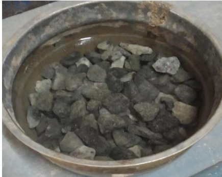
Fig3 Test For Water Absorption Of C.A
