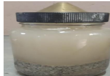
Fig 2 Specific Gravity Test For Coarse Aggregate
