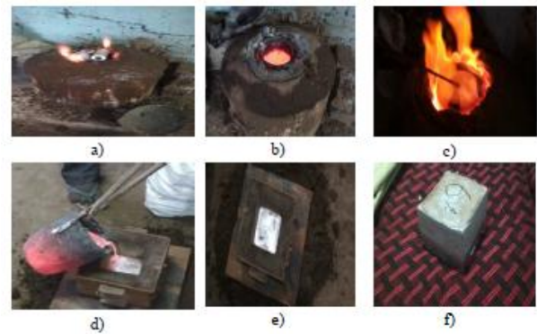
Fig. 1. (a) Al metal heating in furnace (b) Metal comes to a molten state (c) Reinforcement mix with molten metal (d) Pouring molten metal (e) Molten metal kept for cooling (f) Casted part
