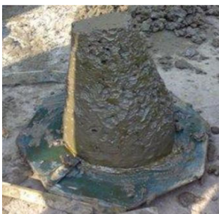
FIG-1: SLUMP CONE TEST
