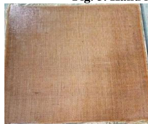
Fig. 4. Laminate of j-g fiber with epoxy resin
