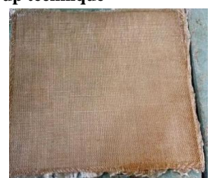
Fig. 5. Laminate of j-g with polyester resin
