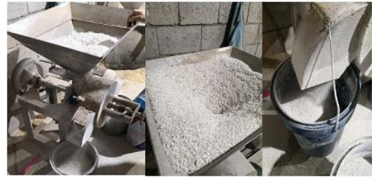
Fig. 3. Secondary crushing using grain milling machine
