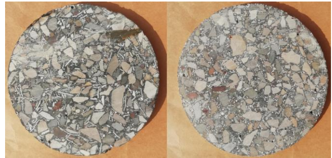
Fig. 8. View of sawed cylinder (a) Concrete with coarse grading plastic (b) Concrete with fine grading plastic
