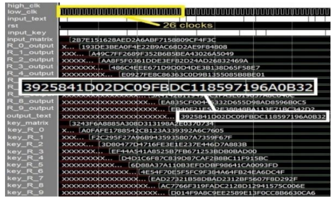
Fig. 12. The ModelSim Simulation of the Normal AES processing
