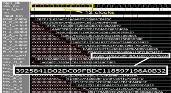
Fig. 13. The ModelSim Simulation of the Pipelined AES processing
