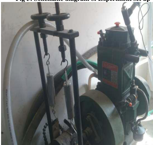
Fig 4: Engine Test Rig
