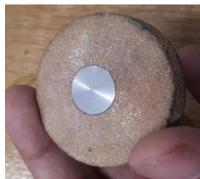
Fig. 5. Composite porous stone for AE study
