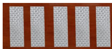
Fig. 1. Glass -epoxy specimens with Si C admixture
