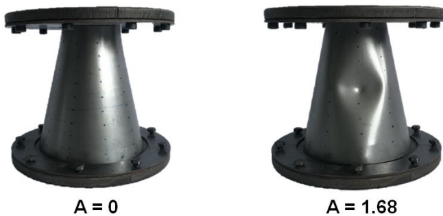
Fig. 4. Experimental setup for conical shells with different imperfection amplitude, A = 1.68.
