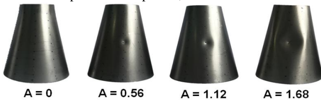
Fig. 2. Typical photograph of conical specimens with different dimple amplitude.
