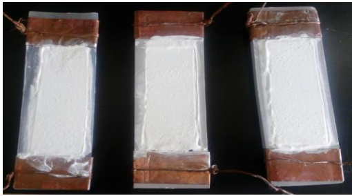
Figure 5. Pollution layer of thickness 0.25 mm using former made according to 2.3
