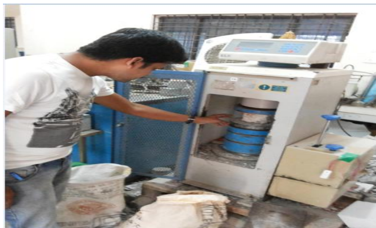
Fig. 4. Compressive Strength Test Setup in CTM
