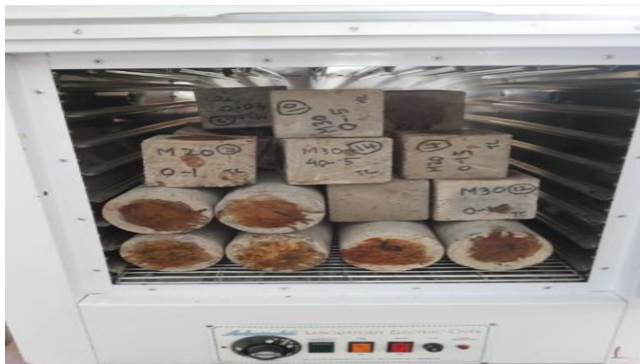
Fig. 5. Concrete Specimens Subjected to Elevated Temperature
