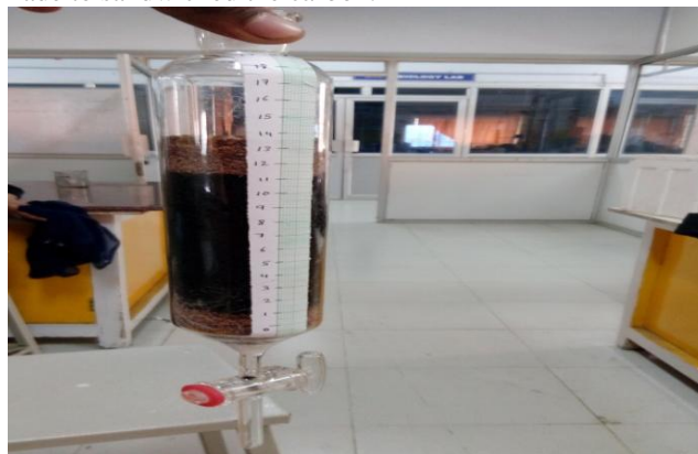
Fig 2. Glass column with sand and carbon particles
