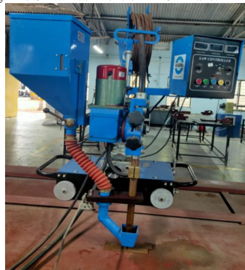
Fig. 2 SAW machine used for experiments
