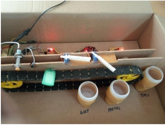
Figure 9: Metal detecting sensor activated, metal waste is segregating to the dustbin
