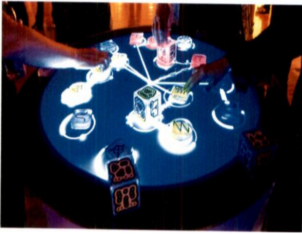
Fig. 1: The Readable: a multitouch interface for playing music
