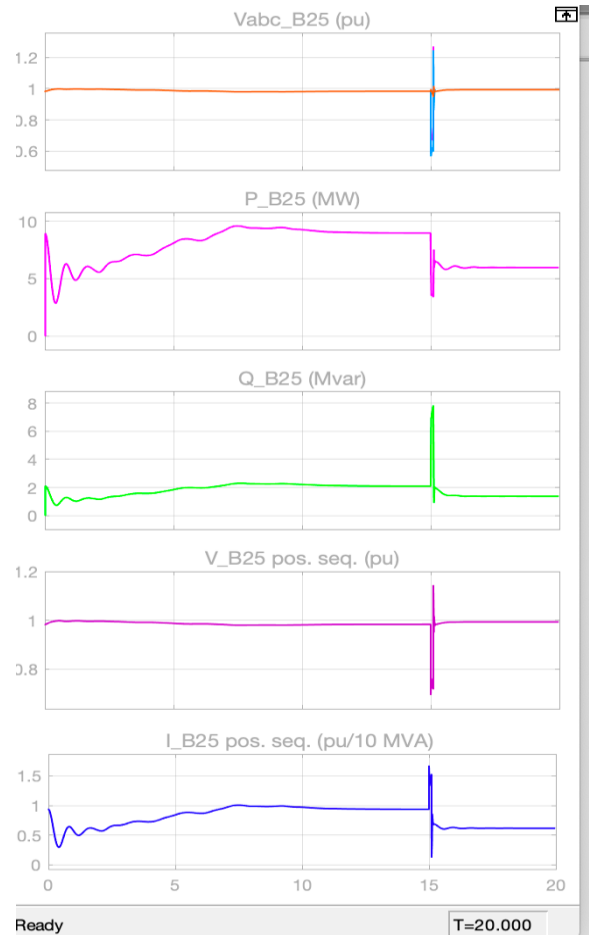
Figure 11. Response at B25 busbar system
