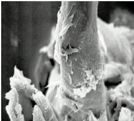
Fig.5 Microscopic view of sisal fibre failed due to tension
