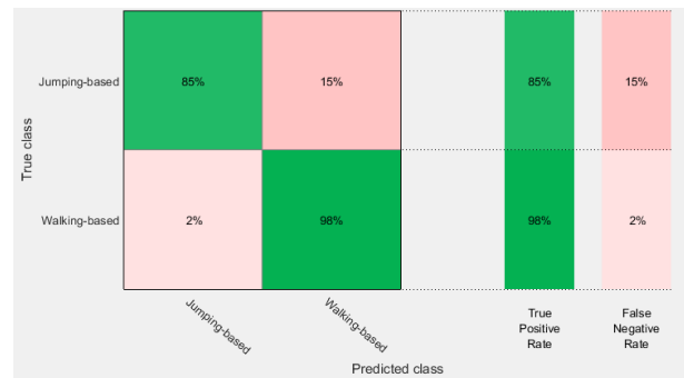
Fig. 9. Confusion matrix (True Positive Rate and False Negative Rate) for k-NN classification model used in this study.
