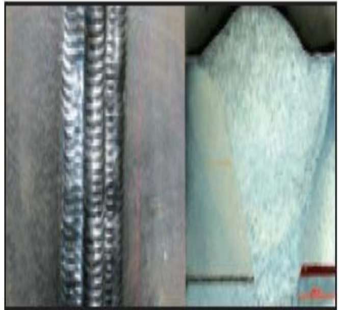
Fig 4. Macroscopic picture of the as-deposited weld bead
