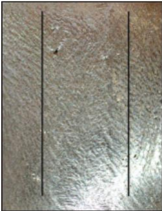
Figure 5 Macroscopic surface of the root bend test sample.
