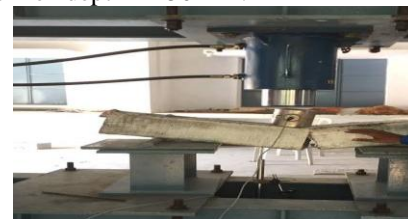
Fig 7: flexural strength test for beam
