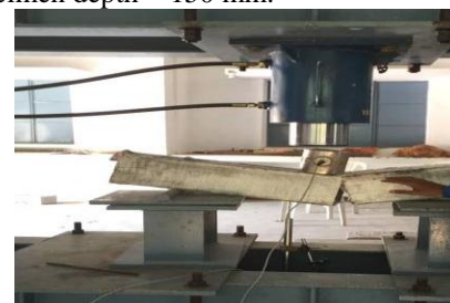
Fig 7: flexural strength test for beam
