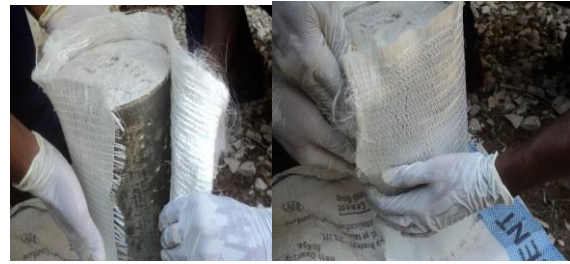
Fig.3 Applying of fiber sheet
