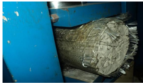
Fig 6: Split Tensile Test on cylinders
