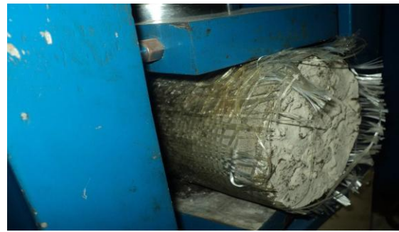
Fig 6: Split Tensile Test on cylinders
