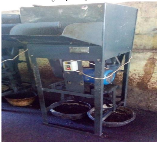
Fig 2. Cashew nut cutting machine
