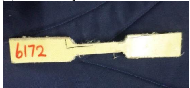
Fig. 7. Specimen prepared for the tensile test
