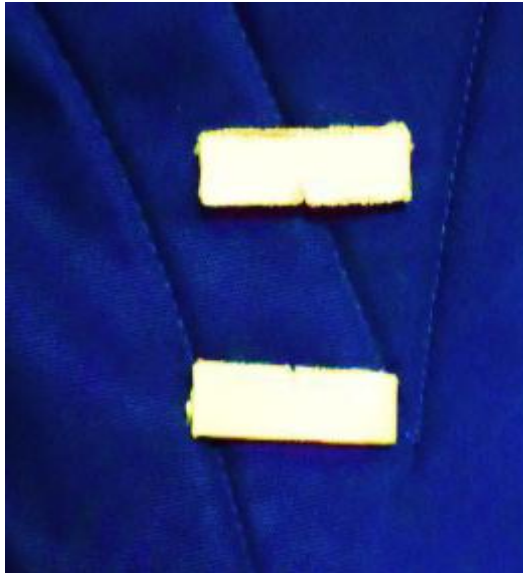
Fig.9. Specimen before impact test
