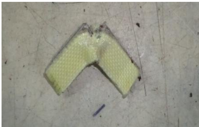
Fig.10. Specimen after impact test
