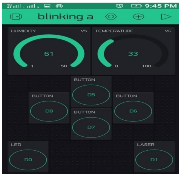
Fig.5. Widget created for controlling Laser shoot, Directional movements, temperature and humidity updates and night vision light by using Blynk.
