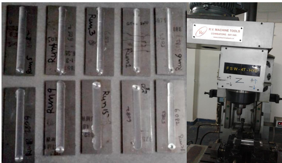
(a) (b) Fig.1. Pictures of few FSW plates and FSW machine
