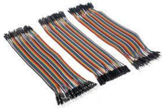
Fig .6. Jumper Wires.
