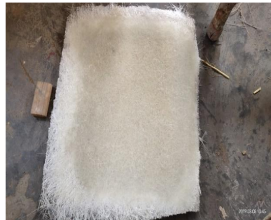
Fig. 1. Composite prepared by Hand layup Process.
