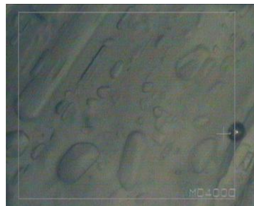
Fig.5 Etch pit pattern of LSS crystal
