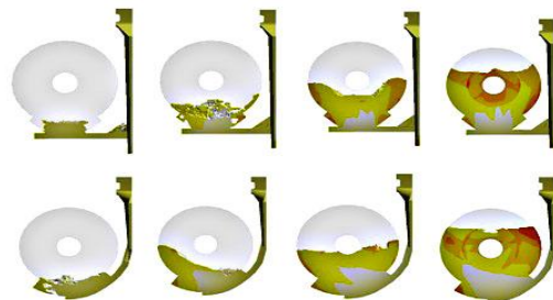
Fig. 7 Various gating design of brake disk filling: conventional (upper) and optimized streamlined gating system (lower) [28].
