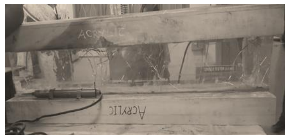
Fig.3 : Crack propagation in Acrylic adhesive specimen
