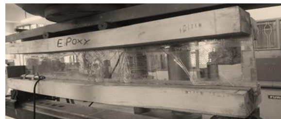
Fig.4 : Crack propagation in Epoxy adhesive specimen
