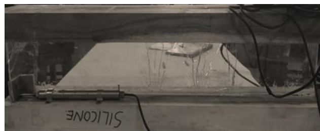
Fig.5 : Crack propagation in Silicone adhesive specimen
