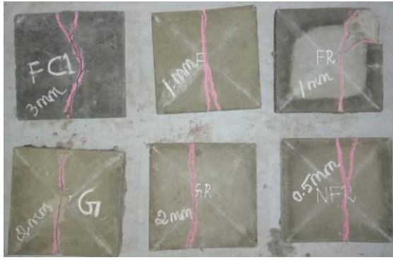
Fig. 8. Crack pattern on bottom surface of panels
