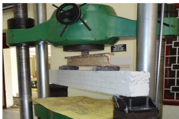
Fig. 2 Test setup of two point loading
