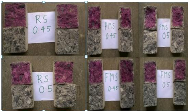
Fig.3.Indication of depth of CO 2 penetrated
