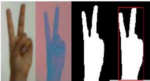
Fig 2. Example: Original image, YCbCr image, binary image and localized hand object
