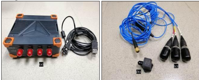
Fig. 3: Measuring equipment; (a) Data acquisition module 4 channel ; (b) triaxial ICP accelerometer ; (c) 4 pin BNC cable
