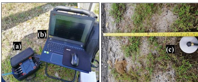
Fig. 4: Measuring equipment arrangement; (a) Data acquisition module 4 channel; (b) Portable computer; (c) Triaxial ICP accelerometer
