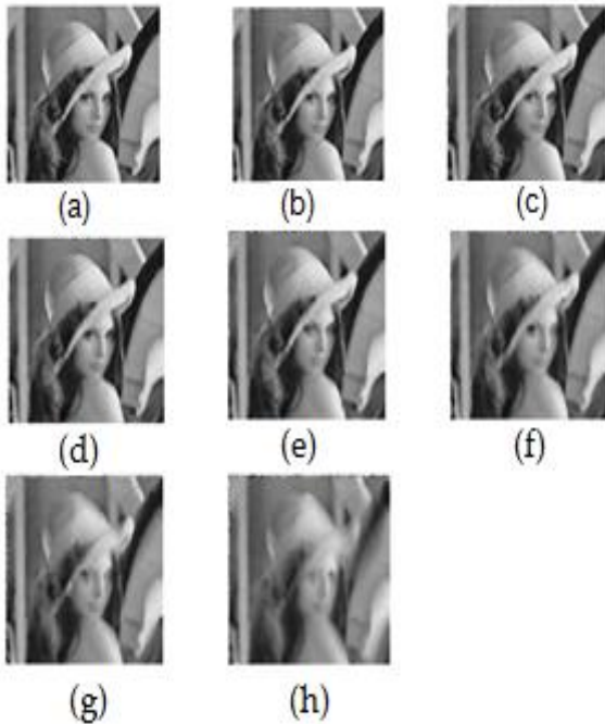
Fig. 10. Results for a 7x7 filter for various noise density values
