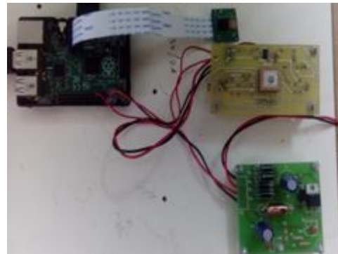
Figure 4.3 Pi with GPS Receiver and Picamera
