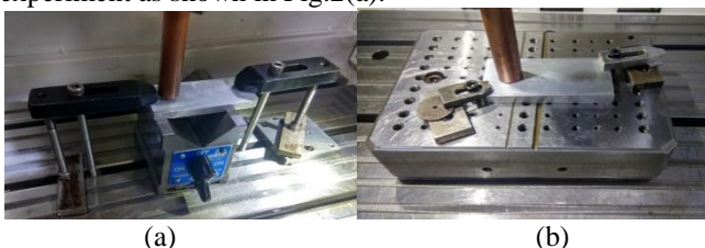
Fig.2 Fixture used for (a) stationary EDM (b) rotary EDM
