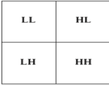
Figure 4: DWT divide's an image into 4 bands; LL, LH, HL and HH.
