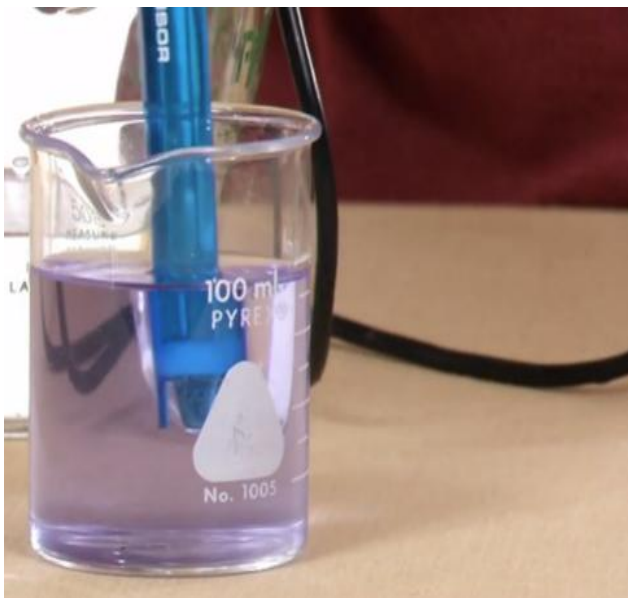
Fig.7:Testing the solution using pH sensor
