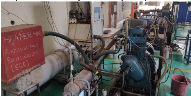
Fig. 1 Modified diesel engine with low pressure petrol injection facility
