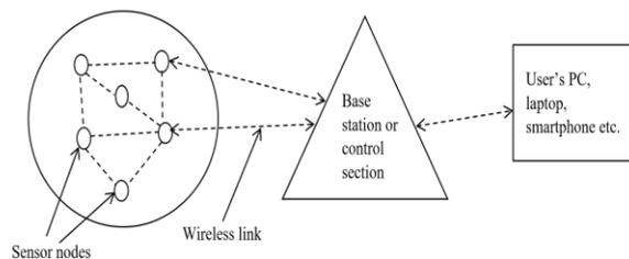
The figure above is the overview of smart agriculture using WSN which is divided into 3 parts: sensor nodes or mote, base station (control section) and the user end consisting of Internet or GSM enabled devices which can receive all the data gathered by the sensors with the help of which a user can analyze the data and hence can act accordingly. The sensors are deployed in the agricultural field.
