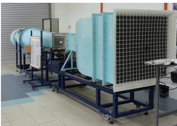
Fig. 4. Wind tunnel used in this study – the test section is located between the two blue sections on the left and right
