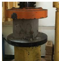
Fig:9 Samples under the compressive strength test
