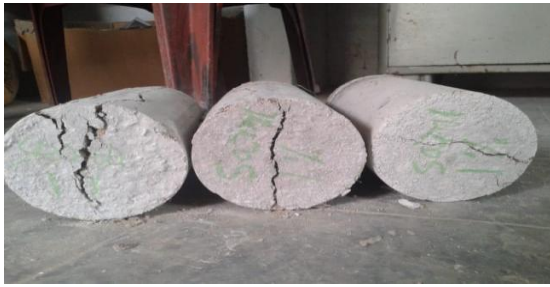
Fig 3: Tested specimens under split tension.
