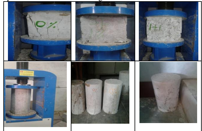
Fig 2: Cube and cylinders under compressive test
