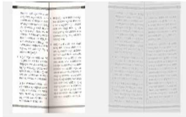
(a) Image with Non-uniform illumination (b) Image with uniform illumination Fig. 4. Results of Local Contrast Normalization on two sided scanned documents
