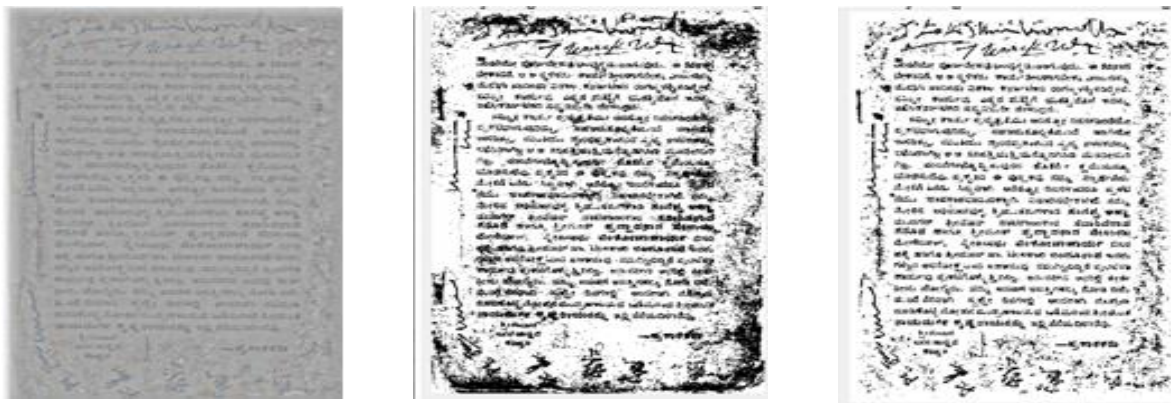
(a) Image after LCN (b) Binarization without Gaussian smoothing (c) Binarization after Gaussian smoothing Fig. 5. Result of Gaussian smoothing
