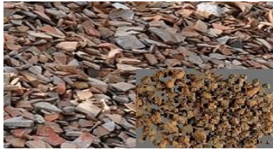
Fig. 1. Crushed Pottery Waste (PW)
